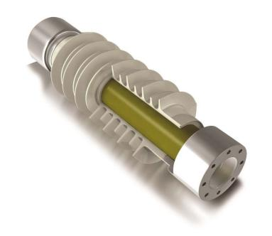
The manufacture of composite insulators is a complex process. The manufacture of the Glass Tube inside the insulator requires a Roving wound Spiral wet winding process, where the Glass fibres are passed through a combination Epoxy formulation to provide a strong, thermally stable and crack free composite tube after curing. Ulticast® resins offer a combination of formulations for Rods and Tubes for Class F & H applications with excellent wetting properties to the glass fibres.
